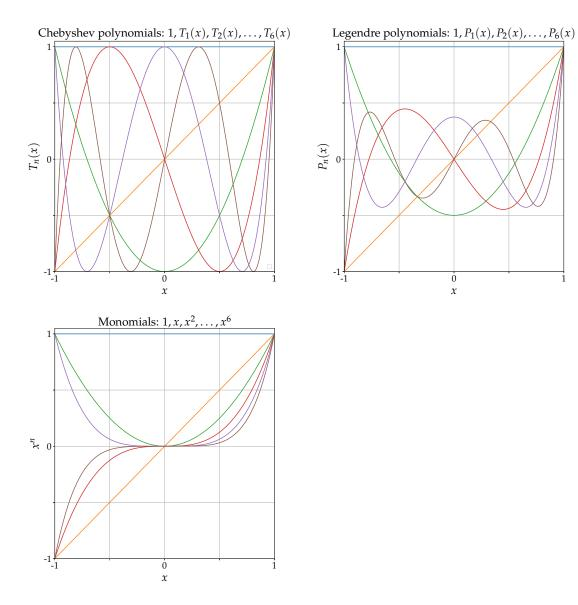
Figure 15.2. The three alternative <polynomial-type>s used to make two dimensional polynomial trend maps. Chebyshev is the default.
