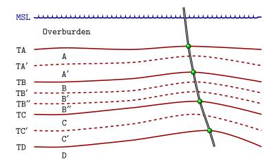
Figure 8.6. A simple set of zones with a zonation finer than the surface model. The well points are given as green bullets.
