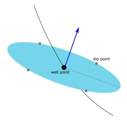
Figure 8.13. Four dip points located on a ellipsoid in the dip plane passing through the well point.
