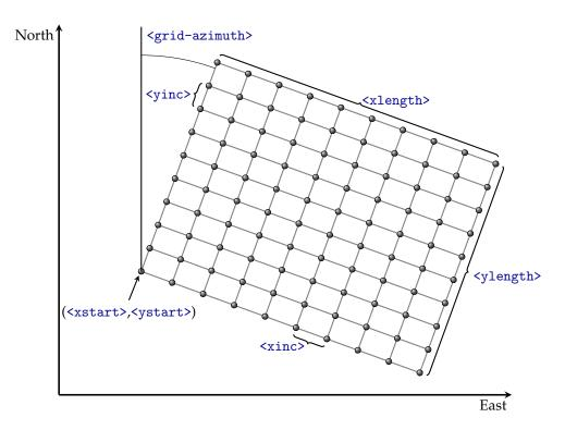
Figure 17.1. Elements used to specify the output grid definition: <grid-azimuth>, <xinc>, <yinc>, <xlength>, <ylength>, <xstart> and <ystart>. Note that using <read-from-file> is simpler. The surfaces are defined at the grid nodes (gray bullets). COHIBA uses bilinear interpolation (Section 20.6.1) to approximate the surfaces inside the rectangles.
