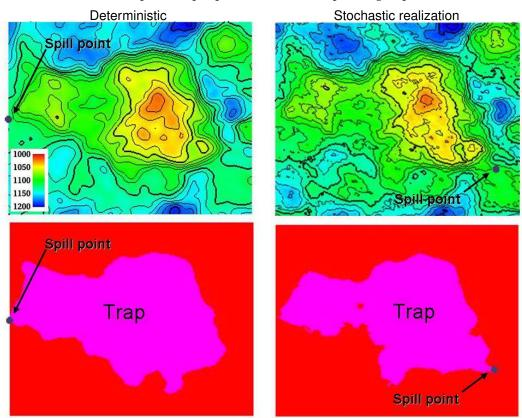
The spill point is detected and written to file (x-, y-, and TVD-coordinate). Also the trapped area can be written to an output grid file. Note that the spill point for the predicted and the simulated surfaces can be quite different.
