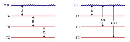
Figure 14.1. Three surfaces, TA, TB, and TC obtained by adding deeper intervals (left) or by attaching them directly to the reference surface MSL.
