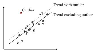
Outliers will often have significant impact on the trends and cause "bulls eyes" in surfaces. Outliers are classified as *outlier*, *severe outlier*, *error* or *extreme error* depending on severity. Outliers are tagged, severe outliers are given a well point TVD pick uncertainty, and errors and extreme errors are excluded from all calculations. See Section 20.3.5.1 for details on how outliers are classified.
