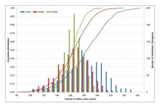
Figure 10.4. Histogram in bins of 8 million cubic meters and cumulative distribution of calculated volumes from 1000 realizations with 1, 2, and 3 wells.
