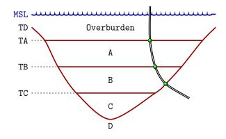
Figure 8.4. Zones where surface TD is onlapped. The well points are given as green bullets.
