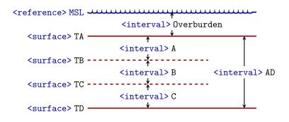
Figure 20.1. Schematic cross section of <surfaces> (TA, TB, TC, TD) and intervals (Overburden, A, B, C, AD). Note that <surface> TA is the <top> for <interval> A and AD, and <surface> TD is the <base> of <interval> D and AD.
