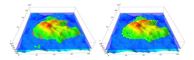
Figure 13.1. Surface constrained by an oil water contact (OWC). Th left figure shows the original surface whereas the right figure shows the surface constrained by the OWC. White points marks sampled locations where the surface is enforced to be above the OWC and black points marks locations where the surface is enforced to be below the OWC.
