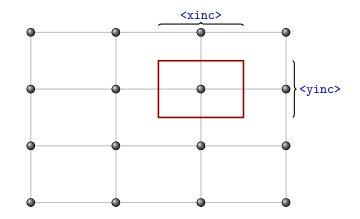
Figure 9.1. The volume within the red rectangle is assigned to the grid node in the center of the red rectangle.
