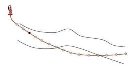
2. Along the well paths, calculate the deterministic surface (solid lines), and the prediction uncertainty (dashed lines) given the well points. This is quite efficient since only a fraction of the grid nodes are close to the well paths.
