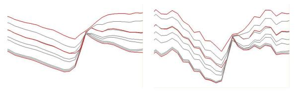
Introducing eroding and onlapped seismic reflectors (Turn off using element <treat-reflectors-as-eroding-and-onlapped>):
