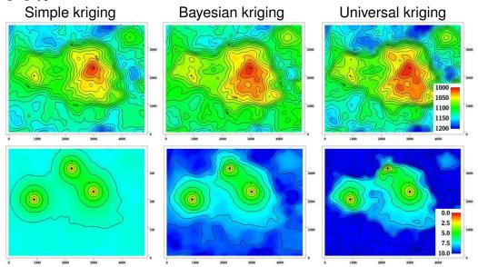
The upper row contains the surface depths and the lower row the corresponding prediction uncertainty. There are two trend coefficients in this example that corresponds to surface
