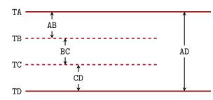
The figure shows a schematic cross section of surfaces (TA, TB, TC, TD) and intervals (AB, BC, CD, AD). Note that surface TA is the top for intervals AB and AD, and surface TD is the base of intervals AD and CD.
