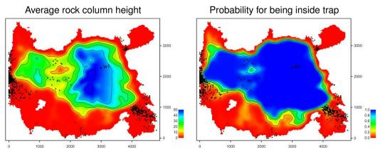
These maps are the average of 1000 realizations. The small black dots are the 1000 different spill points. For an extensive discussion of the possibilities see Section 10.
