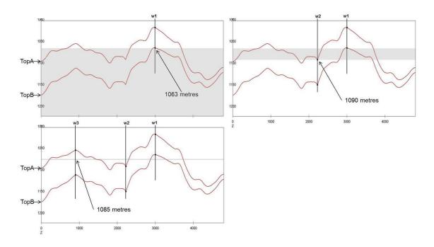
Figure 10.2. Fence diagram through the three wells. The grey areas indicate the acceptable depths for the spill points for the three cases.
