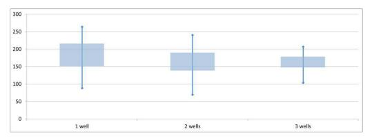
Figure 10.5. Box plot showing statistics of the calculated volumes from 1000 realizations in million cubic meters. The top and bottom of the vertical lines are the maximum and minimum volume. The top and bottom of the rectangle are the average volume plus and minus one SD.
