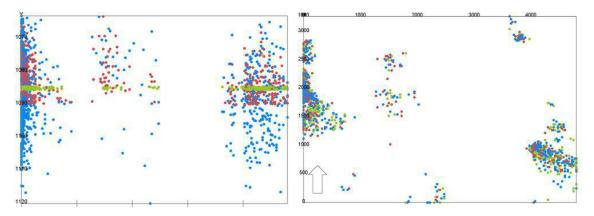
Figure 10.3. Spill points from 1000 realizations with 1, 2, and 3 wells. Left figure is a vertical cross section along the x-direction. The right figure is a top view. Blue spill points are constrained by 1 well, red spill points are constrained by 2 wells, and the green spill points are constrained by 3 wells.
