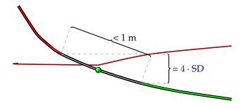
Figure 8.10. Cross section of one surface along a well path. A short ( $\Delta MD \le 1$  meter) undefined zone log section is replaced by a well point (green dot) at the center with TVD pick uncertainty (SD) equal to  $\frac{1}{4} \Delta TVD$ .
